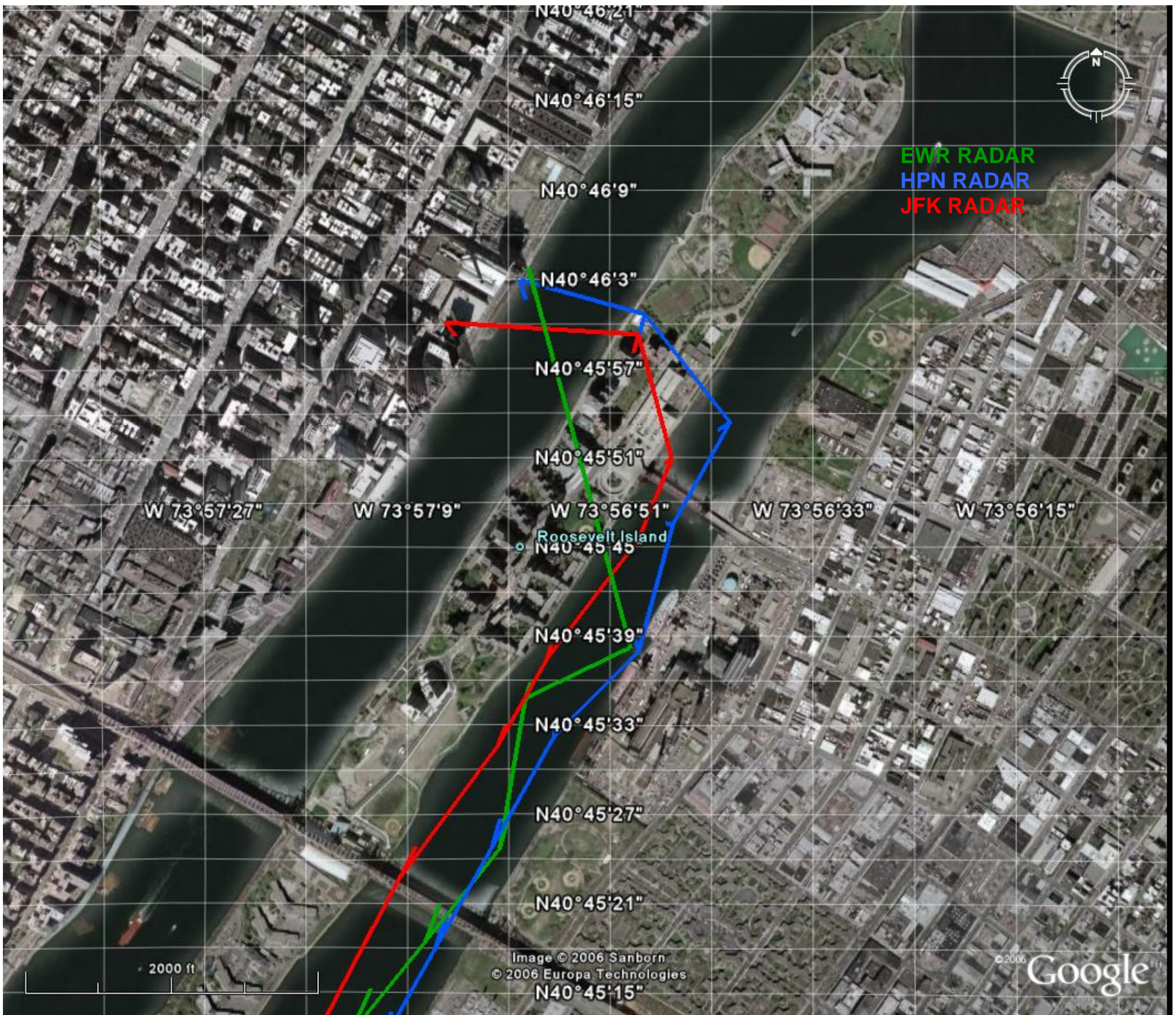
Figure 2: Radar data points from EWR, HPN, and JFK ASR-9 radar sites connected with respective straight line segments, projected to the earth's surface, and overlaid on satellite image (Roosevelt Island is shown in the center of the image).
